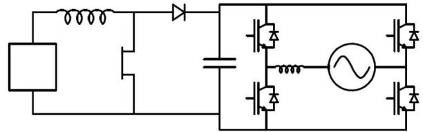
(a) Basic dc link inverter with input boost converter.
