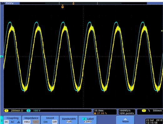
(b) Grid voltage and injected current for inverter delivering active and reactive power.
