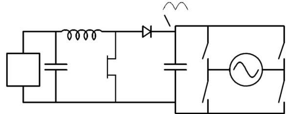
(b) Inverter with variable link to support output unfolding bridge.
