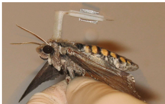
Figure 2: energy harvester attached to Manduca Sexta . Courtesy of WM Tsang, MIT.
