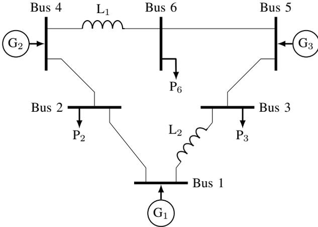
Fig. 4. One line diagram of small-footprint power system
