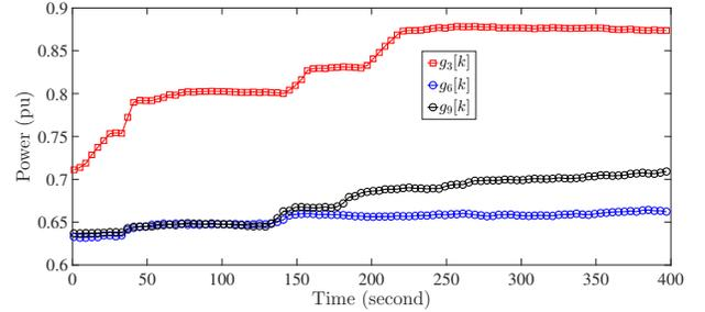
Fig. 4. The output of the DERs  $g_3[k]$ ,  $g_6[k]$ , and  $g_9[k]$  as a function of time.
