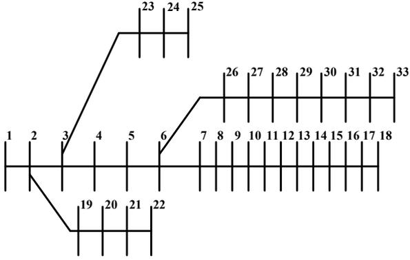
Fig. 2. A grid-connected microgrid comprising three generator buses, 29 load buses, and one tie-line bus.
