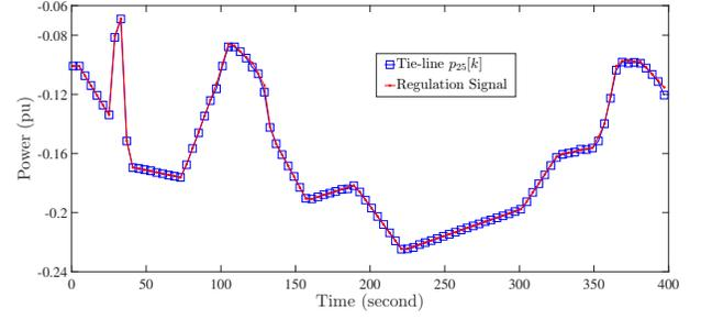
Fig. 3. Power exchange  $p_{25}[k]$  and regulation signal  $r[k]$  as a function of time.
