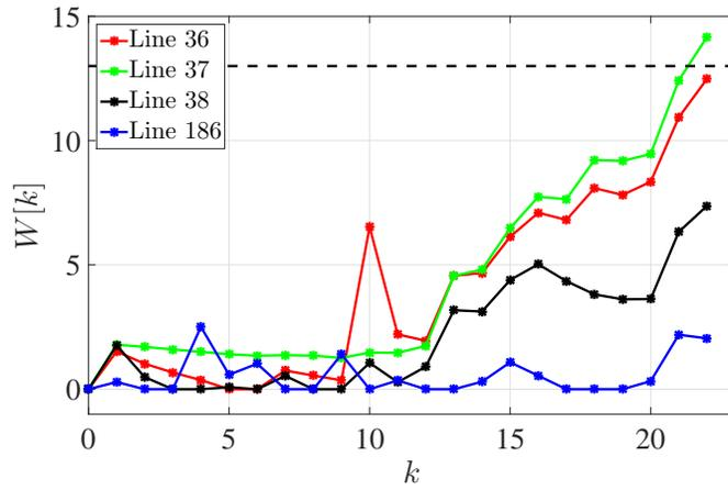
(b) Line 36 outage with  $b=13$ .**Figure 1.2** Sample paths of the G-D-CuSum algorithm for IEEE 118-bus test system.
