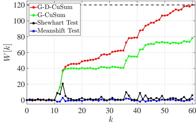
(a) Line 180 outage with  $b=120$ .
