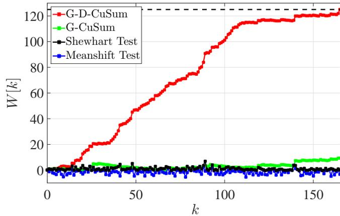
(b) Line 32 outage with  $b=125$ .**Figure 1.1** Sample paths of different algorithms for IEEE 118-bus test system.
