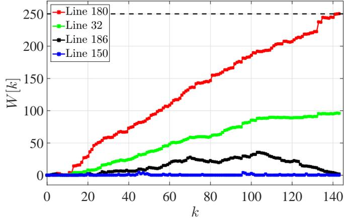
(a) Line 180 outage with  $b=250$ .
